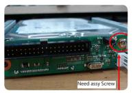
3. Select "Master" or "Slave" using the Jumper switch on SATA converter board. Set the Master/Slave using the Jumper switch.
